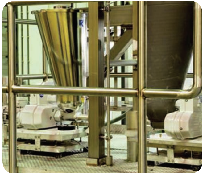
Automated dosing feeders ensure ingredients are added in the correct ratio by controlling the material feed rate, by weight.
